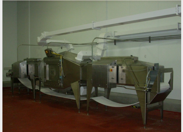
CT-150 with 2X75Kw WaveGen Power Supplies (out of view)
